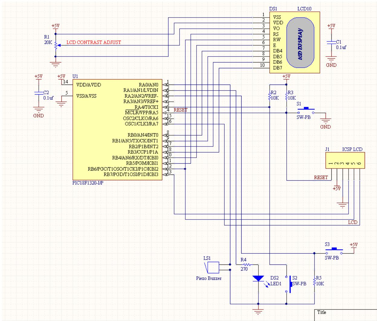
Here is the schematic for the PIC18F1320 LCD Demo.
